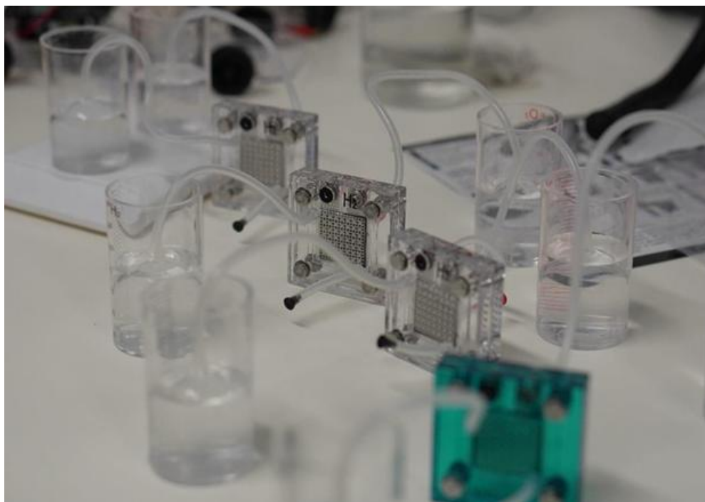
Figure 2. 1 Multi Reversible Fuel Cell Stack. (Sundaresan et al. (2020))
